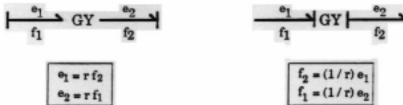
Figure 7.22. Causality bond graph for the ideal gyrator
