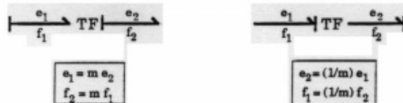
Figure 7.20. Causality bond graph for the ideal transformer
