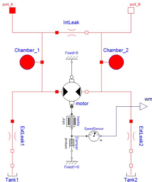
Fig.5: Hydraulic motor
