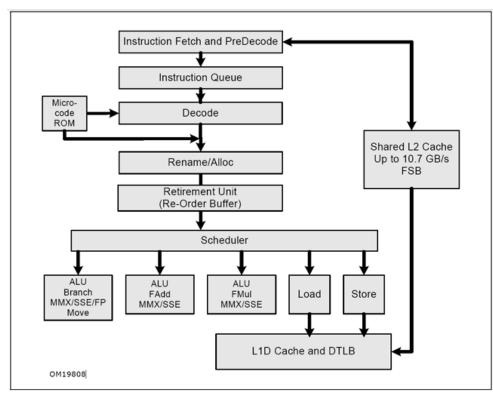
Figure 2-1. Intel Core Microarchitecture Pipeline Functionality
