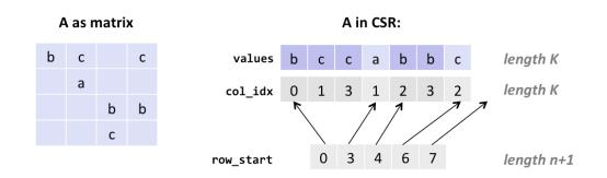
Figure 1: Compressed sparse row (CSR) format.
