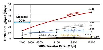
Figure 13: Throughput of DRAM-based TRNGs projected on DDR4 transfer rate. We plot transfer rates beyond the DDR4 standard [76].
