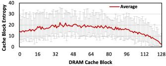
Figure 10: Average entropy of each cache block in the highestentropy segment in all modules. The error bars show the range of the values across all modules.
