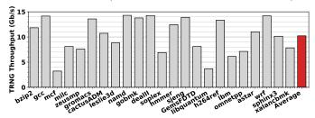
Figure 12: Available TRNG throughput during idle DRAM cycles while running SPEC2006 workloads.
