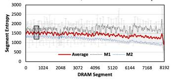
Figure 9: Average DRAM segment entropy across 17 modules (136 chips). The X-axis plots the DRAM segments and the Y-axis shows the segment entropy. We plot the segment entropy of two specific modules (M1 & M2) using black (dotted) and blue (dashed) lines.
