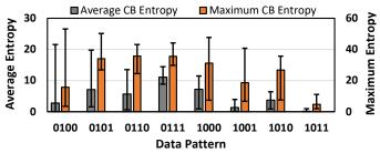
Figure 8: Average (grey bars, left Y-axis) and maximum (orange bars, right Y-axis) DRAM cache block entropies for different data patterns across 17 modules. The error bars show the range of the average and the maximum DRAM cache block entropy across all modules.
