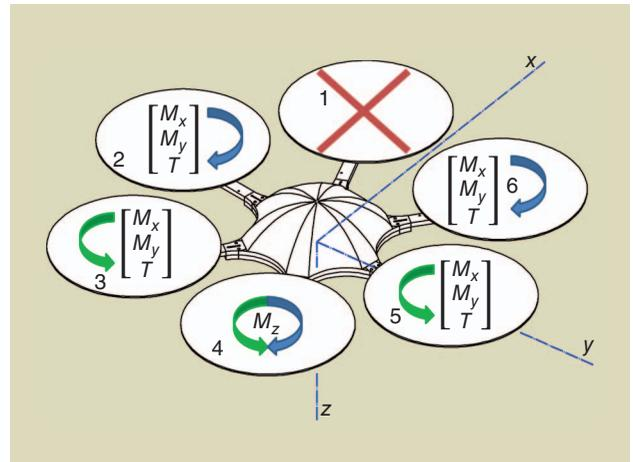
**Figure 2.** This illustration shows the redundancy against single-rotor failure. Assuming that motor 1 is failing, motors 2, 3, 5, and 6 are controlled by the thrust command and the roll and pitch controllers' output. Motor 4—on the opposite side of the failing motor—compensates and controls the yaw momentum by repeatedly changing its direction.
