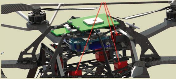
**Figure 4.** The computer-aided design (CAD) model illustrating the vibration damping between the two parts of the frame: the motors and the landing gear are connected to the outer frame, and the inner frame to the IMU, battery, and payload. The silicon dampers are highlighted in red.
