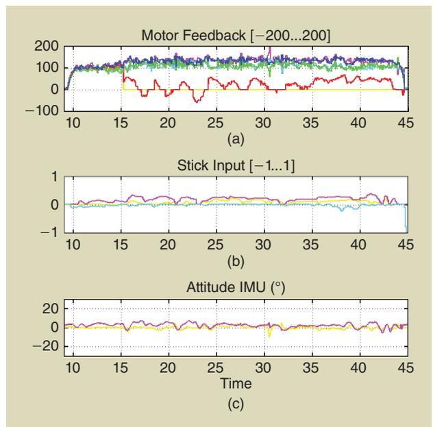
**Figure 12.** (a) The motor commands in a range  $[-100, 200]$  are shown. At about 14 s, the yellow motor is disabled so that the redundancy controller can be activated. As observed, the red motor command slowly oscillates around zero to compensate for the yaw moment. (b) and (c) There is nearly no influence of the failing motor to the pilot's commands or the measured attitude.
