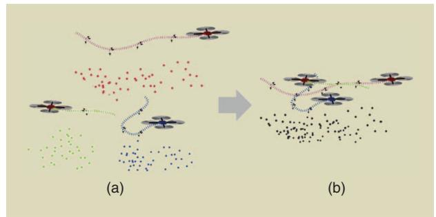
**Figure 7.** (a) The local-navigation module (running on board) estimates the pose of each MAV independently for each platform. (b) The global-navigation module (offboard) recognizes path intersections and uses them to express the MAVs' poses in the same, global coordinate frame and to reduce drift.
