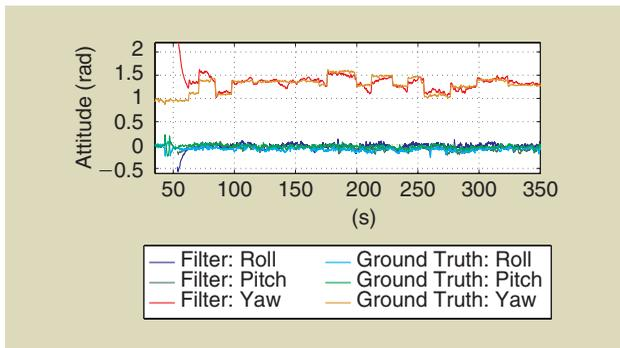
**Figure 14.** A comparison between EKF-based attitude estimate (filter: roll, pitch, yaw) and GPS-IMU based estimates from the AscTec internal state estimator (ground truth: roll, pitch, yaw) during a 5-min interval of time.
