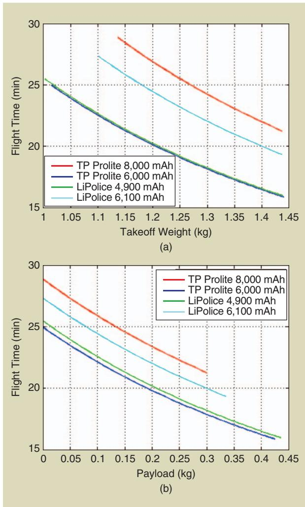
**Figure 6.** The calculated flight time is plotted versus (a) takeoff weight and (b) payload. The estimated flight time for a given payload with different batteries is shown. Thunder Power (TP) and LiPolice are LiPo battery manufacturers.
