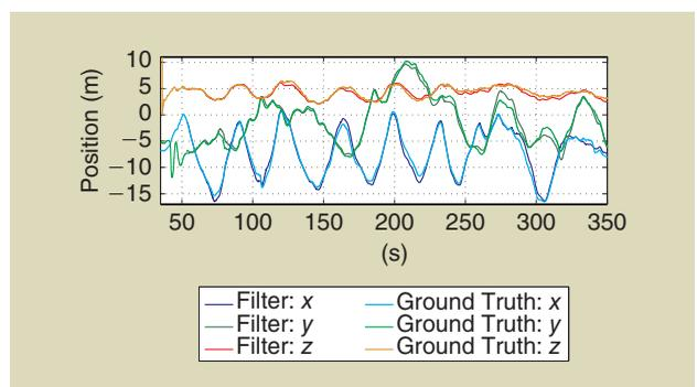
**Figure 13.** A comparison between EKF-based position estimate (filter:  $x, y, z$ ) and raw GPS measurements (ground truth:  $x, y, z$ ) during a 5-min interval of time. The plot suggests that the absolute scale is estimated correctly.
