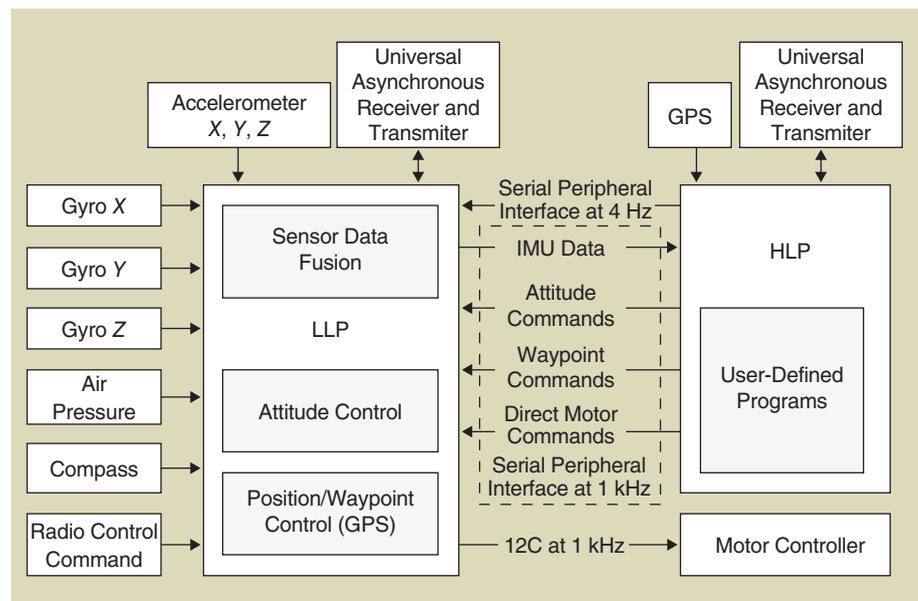
**Figure 3.** The electronic architecture: all sensors, except the GPS, are connected to the LLP, which communicates via I2C with the motor controllers and via the serial peripheral interface with the HLP. For this article, position control and state estimation for local navigation are implemented in the “user-defined programs” section of the HLP (see Figure 8). The position (waypoint) controller on the LLP is not used here since we work in GPS-denied environments.
