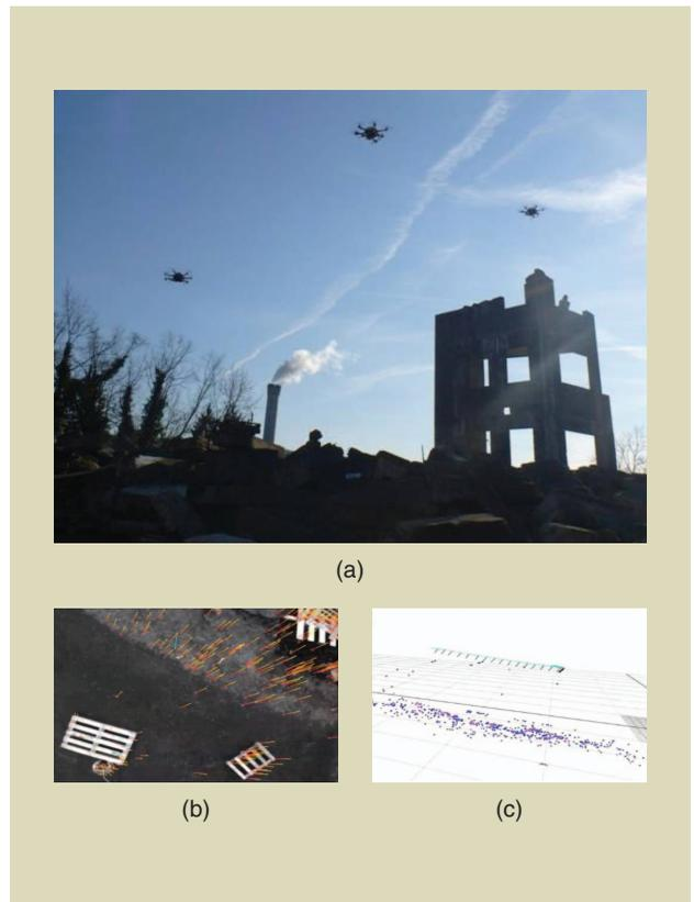
**Figure 16.** (a) The SFLY helicopters during a demonstration of autonomous exploration at the firefighters' training area in Zürich, (b) feature tracks, and (c) the online-built 3-D sparse map used for local navigation.
