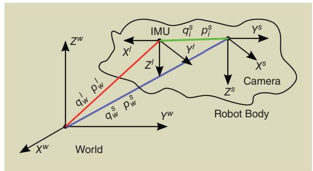
**Figure 9.** A setup depicting the robot body with its sensors with respect to a world reference frame. The system state vector is  $X = \{p_w^i, v_w^i, q_w^i, b_a, b_g, \lambda, p_w^s, q_w^s\}$ , whereas  $p_w^s$  and  $q_w^s$  denote the robot’s sensor measurements in (a possibly scaled) position and attitude, respectively, in a world frame.
