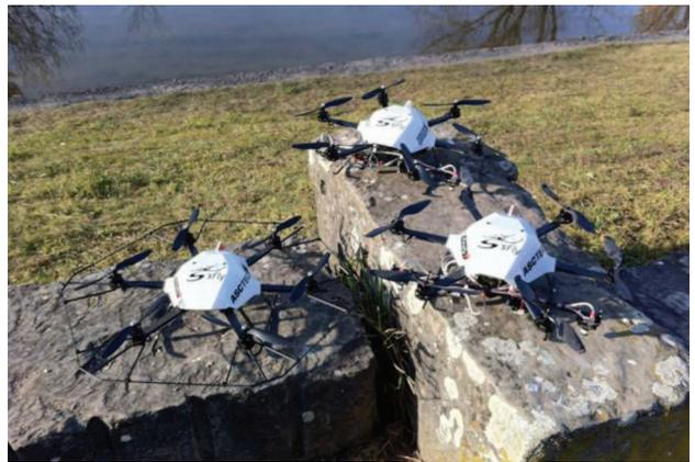
**Figure 1.** The three SFLY hexacopters are designed for inertial-visual navigation in GPS-denied environments.
