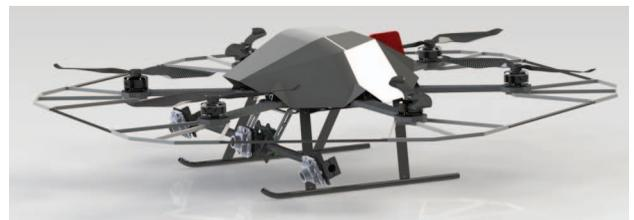
**Figure 5.** The complete CAD model, including three cameras on the SFLY hexacopter.
