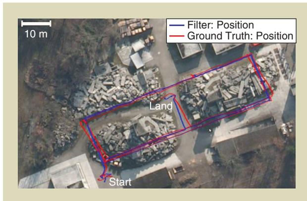
**Figure 15.** After a short initialization phase at the start, vision-based navigation (blue) was switched on for successful completion of a more than 350-m-long trajectory, until battery limitations necessitated landing. The comparison of the estimated trajectory with the GPS ground truth (red) indicates a very low position and yaw drift of the real-time onboard visual odometry.
