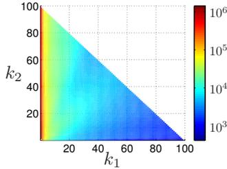
Figure 1. The number of test samples from our large scale data set that hit a certain proportion  $(k_1, k_2)$  during the classification process. The number of samples is color coded on a logarithmic scale.
