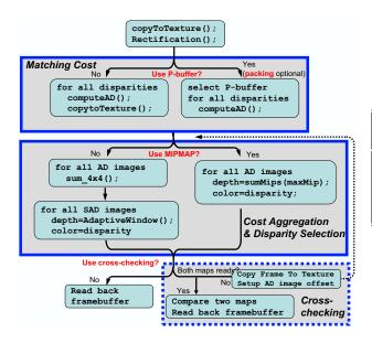
Figure 5: A block diagram of our implementation.
