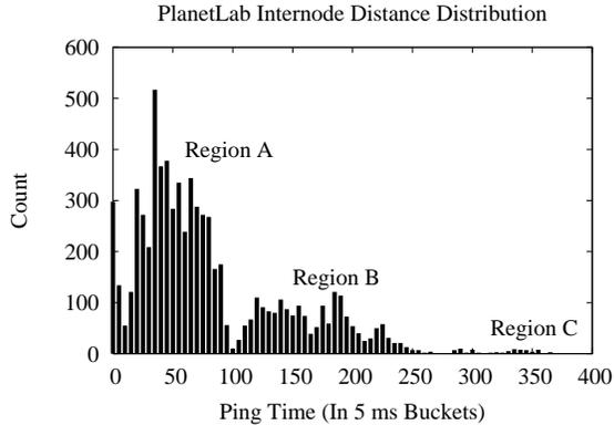
Figure 2: *Distribution of round-trip times in PlanetLab.* Region A (0–100 ms) contains 72.3% of the times, Region B (100–275 ms) contains 26.6%, and Region C (275–400 ms) contains the the negligible remainder.
