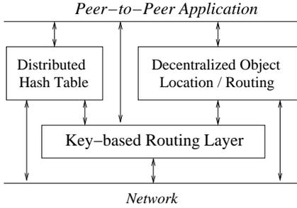
Figure 1: *Overlay Service Decomposition*. The functionality exposed by structured peer-to-peer overlays can be divided into a mapping of keys onto nodes, mechanisms to store and retrieve data items, and mechanisms to route to or locate data items stored according to a policy outside the overlay’s control.
