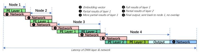
Fig. 5. Overlapping computation and network in a pipelined and parallelized method.
