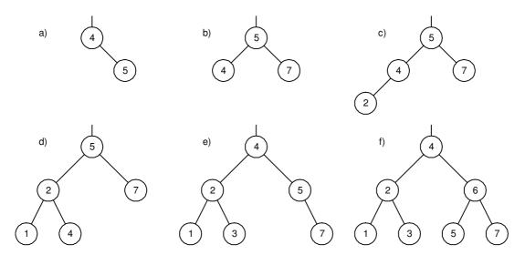
Fig. 4.34. Insertions in balanced tree
