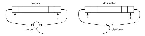
Fig. 2.12. Straight merge sort with two arrays
