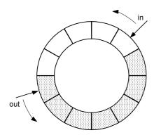
Fig. 1.8. Circular buffer with indices in and out.
