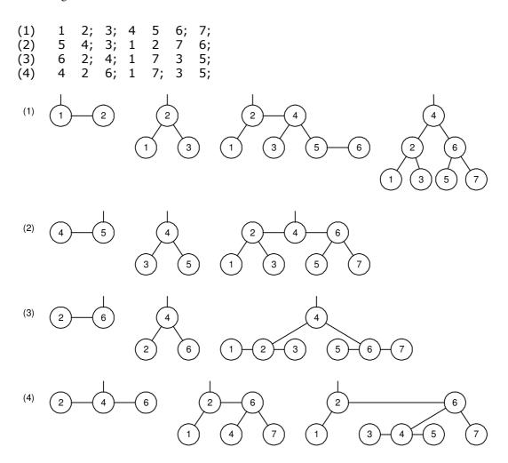
Fig. 4.50. Insertion of keys 1 to 7
