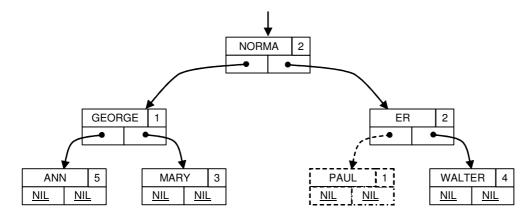
Fig. 4.26. Insertion in ordered binary tree
