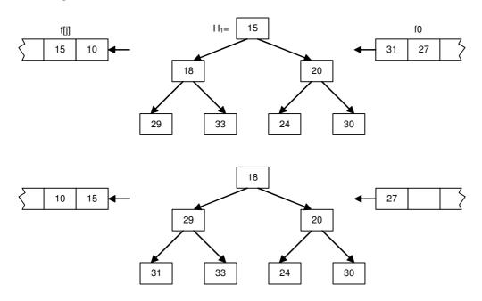
Fig. 2.17. Sifting a key through a heap
