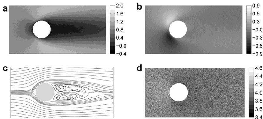
Fig. 10. DPD simulations of the flow past a circular cylinder at  $Re = 40$ . The steady state velocity components: (a)  $u$  and (b)  $v$  indicate that the flow is separated, which is confirmed by the streamlines shown in (c). A uniform density field (d) is observed at the solid walls, and with small variations in flow reflecting the variation in pressure.
