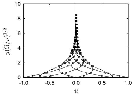
Fig. 7. Stokes flow near an oscillating flat plate: We show the velocity profiles at eight instances during the period:  $t = 2k\pi/8$ ,  $k = 0, \dots, 7$ . DPD simulations are indicated with squares, analytic solutions with lines.
