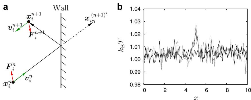
Fig. 1. Sketch of the bounce-forward reflection mechanism. (a) A particle leaving the simulation domain is reinsert using specular reflection, but with inverted velocity and force components. The bounce-forward scheme imposed at a hard wall located in the middle ( $x = 5$ ) of a periodic system ( $\rho = 3$ ,  $a = 25$ ,  $\sigma = 3$ ,  $k_B T = 1$ ) introduces anisotropic perturbations in the fluid temperature. (b)  $k_B T_x$  (—);  $k_B T_y$  (---);  $k_B T_z$  (· · ·).
