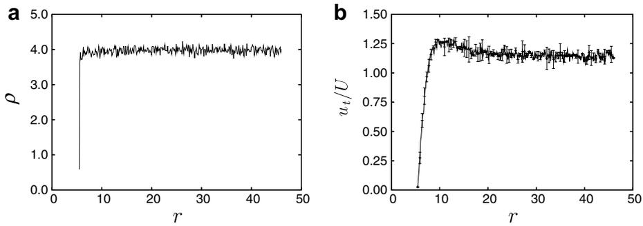
Fig. 9. DPD simulations of the flow past a circular cylinder at  $Re = 40$ . The extracted radial density profile (a) is uniform throughout the system. The corresponding tangential velocity profile ( $u_t/U$ ) is found to satisfy the no-slip condition at the wall and to reach a uniform velocity  $u_t/U \approx 1.14$  in the free stream. The error bars in the velocity are obtained from the measured variation in the velocity in the planes below and above the cylinder cf. Fig. 8.
