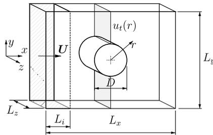
Fig. 8. DPD simulations of the flow past a circular cylinder. (a) Schematic of the simulation setup. The cylinder of diameter  $D$  is placed in the center of the computational box of size  $(L_x, L_y, L_z)$ . A uniform velocity profile with mean  $\mathbf{U} = (U, 0, 0)$  is imposed to particles in the inlet region of size  $L_i$ . Radial profiles of the tangential velocity and density are extracted in the vertical plane intersecting the center of the cylinder (shaded area).
