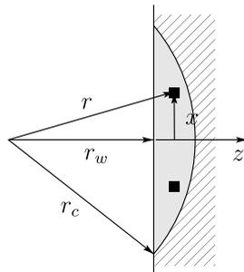
Fig. 3. Integration domains for effective boundary forces.  $r_c$  is the cutoff distance and  $r_w$  the distance to the wall. The normal force contributions along  $z$  are integrated over the shaded area using polar coordinates, the tangential force contributions along  $x$  using cartesian coordinates.
