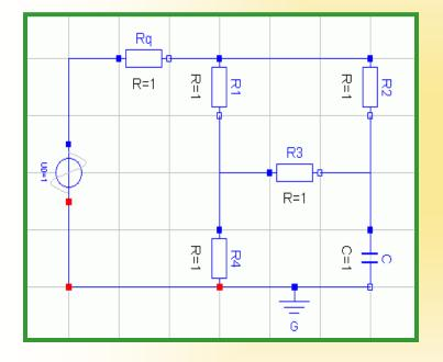
Given the electrical circuit of the figure on the left, determine a complete set of equations in currents and Voltages (by use of both node and mesh equations).
