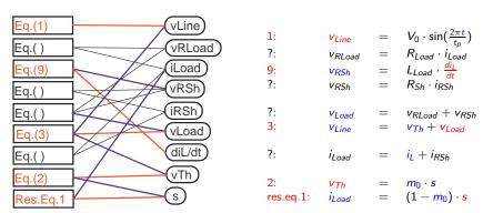
We end up with a second algebraic loop in four equations and four unknowns.
