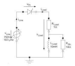
A shunt resistor was added to avoid having to deal with a variable structure model.
