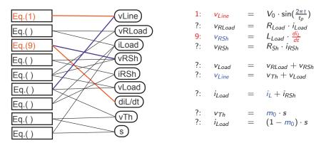
We end up with an algebraic loop in seven equations and seven unknowns. The switch equation (variable s) is part of the loop.
