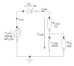
A shunt resistor was added to avoid having to deal with a variable structure model.
