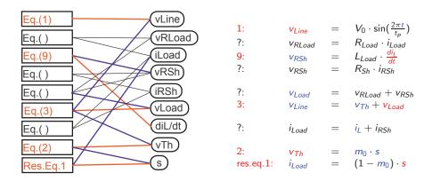
We end up with a second algebraic loop in four equations and four unknowns.
