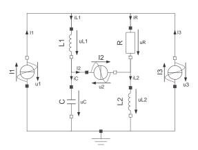
Given the circuit shown below containing three sinusoidal current sources:
