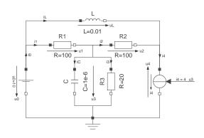
► The circuit contains a constant voltage source,  $u_0$ , and a dependent current source,  $i_4$ , that depends on the voltage across the capacitor, C, and the resistor,  $R_3$ .
