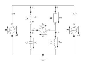
▶ Write down the complete set of equations describing this circuit. Draw the structure digraph and begin causalizing the equations. Determine a constraint equation.
