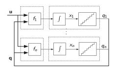
We can model a generic time-invariant quantized system using DEVS models of the static function and quantized integrator types.
