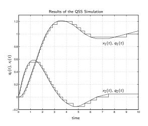
The trajectories of the *state* variables  $x_i(t)$  are *piecewise* linear.
