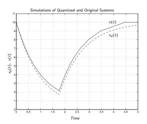
Clearly, the quantized system is a discrete system. However, it cannot be represented by a set of difference equations, i.e., it is not a discrete-time system.
