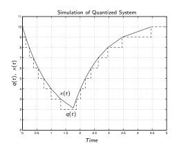
► We were able to complete the simulation in 17 very simple steps, thereby obtaining the exact solution of the quantized system.
