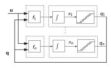
As before, the QSS can be subdivided into *static functions* and *quantized integrators*.
