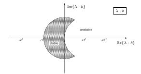
Figure: Numerical stability domain of *predictor-corrector FE-BE technique*
