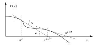
Figure: Newton iteration on a single zero-crossing function
