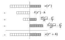
Figure: Effects of the *roundoff error* in 1.5-fold precision
