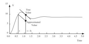
Figure: Numerical integration using the "BE" method
