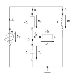
2:  $u_1 = R_1 \cdot i_1$ 3:  $u_2 = R_2 \cdot i_2$ 4:  $u_L = L \cdot \frac{di_L}{dt}$ 5:  $i_C = C \cdot \frac{du_L}{dt}$ 6:  $u_0 = u_1 + u_1$ 7:  $u_L = u_1 + u_2$ 8:  $u_C = u_2$ 9:  $i_0 = i_1 + i_L$ 10:  $i_1 = i_2 + i_C$
