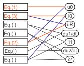
The constraint equation has indeed disappeared. After partial causalization of the equations, we are now faced with an algebraic loop in four equations and four unknowns, a situation that we already know how to deal with.
