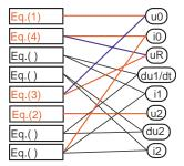
We are again faced with an algebraic loop in four equations and four unknowns.
