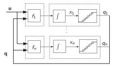
As before, the QSS can be subdivided into *static functions* and *quantized integrators*.
