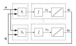
We can model a generic time-invariant quantized system using DEVS models of the static function and quantized integrator types.
