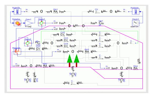
Each 0-junction together with its associated capacitance represents a thermal storage and one temperature value. Different storages represent the soil, the vegetation, the pond, the dome, and the inside atmosphere. Conduction and radiation are modeled in the usual fashion (Cellier 1991), representing the thermal interactions between these thermal storages.
