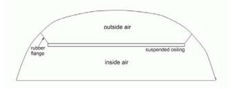
In the model, the Biosphere 2 system is simplified to a single biome, exhibiting the same temperature and humidity throughout the atmosphere, and all material flows (air flow and water flow) were omitted, in order to be able to describe the system by regular bond graphs:
