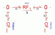
There are two capacitive fields, CF, that store the state variables of the water and of the water vapor, respectively, i.e., entropy, volume, and mass. They compute the three potential variables (efforts): temperature, pressure, and Gibbs potential. The evaporation process, on the other hand, is described by a resistive field, RF, that computes the flows in and out of the two storages, such that the total power into the resistive field equals the total power out of the resistive field.
