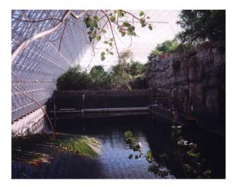
This inside view shows the pond, the high savannah (above the artificial rocks to the right), and the salt water marshes (mangroves) in the background. The glass panels let, on average, pass 60% of the solar radiation, whereas 20% are absorbed by the glass panels, and the remaining 20% are reflected. The pond is about 5m deep, and houses a variety of salt water fish and even a corral reef. Artificial tides were introduced to keep the mangroves healthy.
