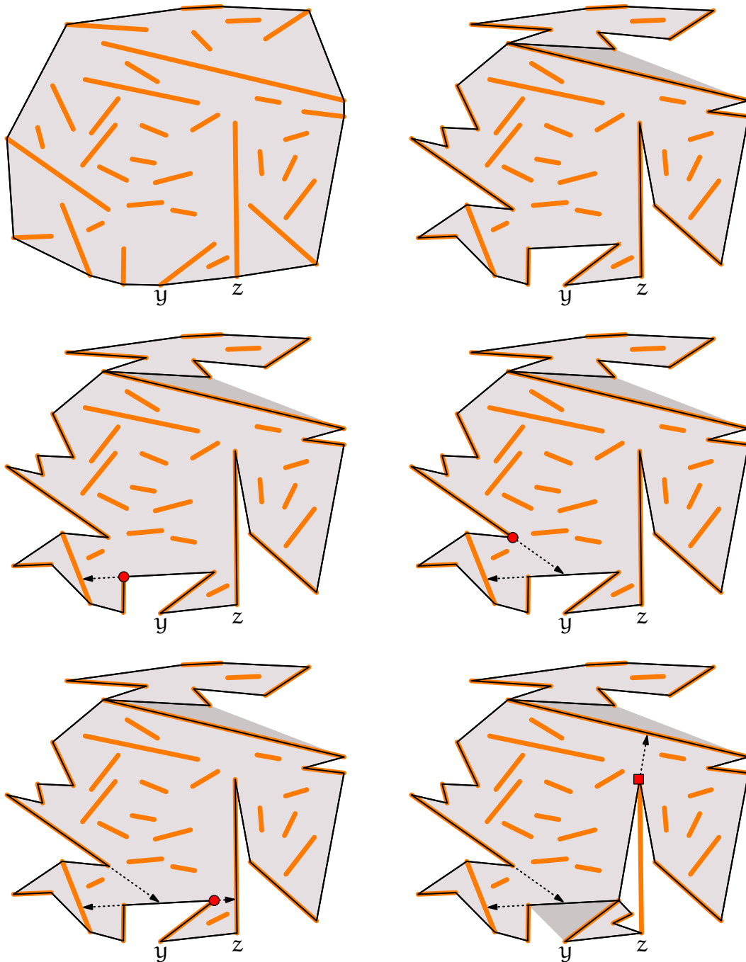
Figure 41: Running Algorithm 3.37 on an example; wedges are shaded dark, and the points from which a ray is shot are marked: a circle denotes a cap, while a square stands for an anti-cap.
