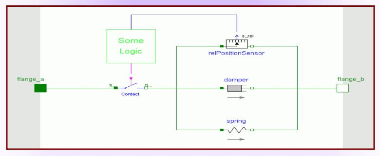
• When the train engine makes contact with the buffer-stop, the switch closes, and the spring/damper system becomes active.
