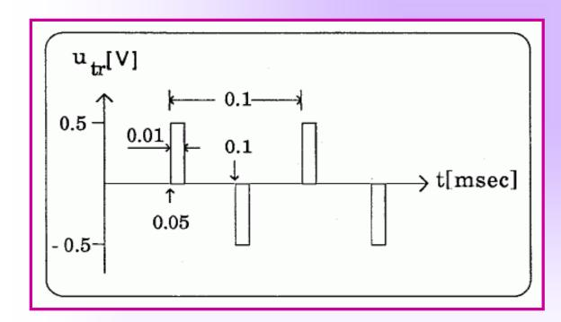
• You can easily create the trigger voltage out of the superposition of two of the pulsed voltage sources provided in the standard bond graph library.
