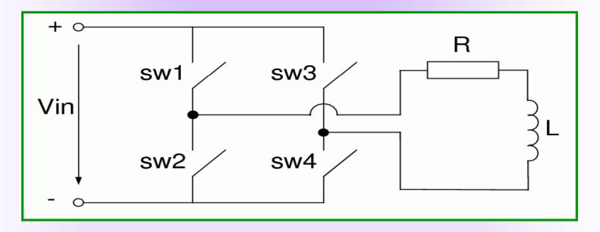
• The purpose is to create an inductor current that is approximately sinusoidal.
