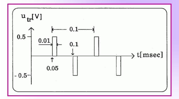
You can easily create the trigger voltage out of the superposition of two of the pulsed voltage sources provided in the standard bond graph library.
