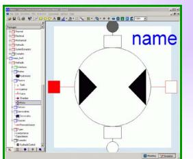
• The motor (screw) model converts hydraulic power into (induced) rotational mechanical power. It can be represented as a transformer.
