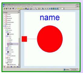
• The chamber model represents a chamber filled with a compressible fluid, usually oil. It can be represented by a capacitor.
