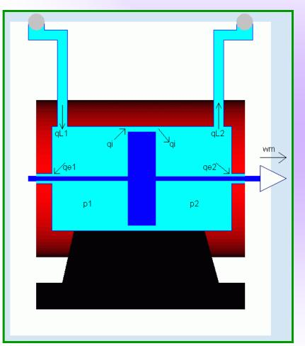
The hydraulic motor has two chambers filled with oil. A wall separates them.
