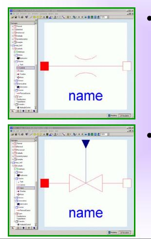
• The laminar resistance model is equivalent to the electrical conductor model. It calculates the flow as a function of the pressure drop.
