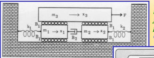
The cutting forces are represented by springs and friction elements that are placed between bodies at a 0-junction.
