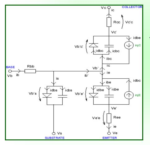
**SPICE** models the BJT by three junction diodes, one from the base to the collector, the second from the base to the emitter, and the third to the substrate.
