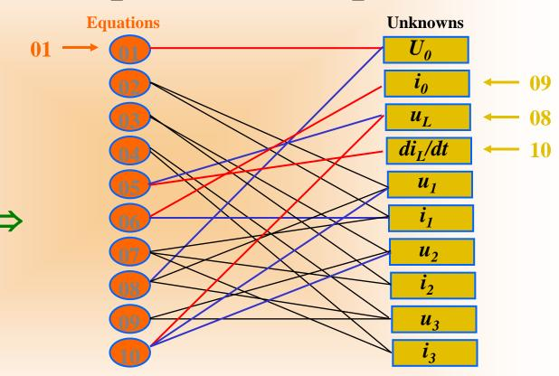
The algorithm stalls, because there are no more single black lines attached to either equations or variables.
