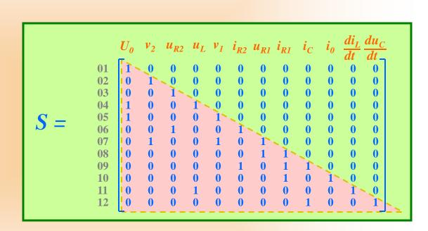
⇒ The structure incidence matrix of the completely sorted equation system is a matrix in lower triangular (LT) form.
