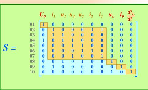
**⇒** The structure incidence matrix assumes the form of a block lower triangular (BLT) matrix.
