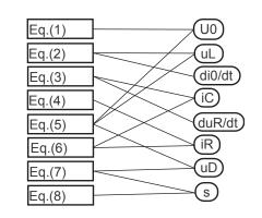
As expected, variable s does not show up inside an algebraic loop. It must be computed from the last equation.
