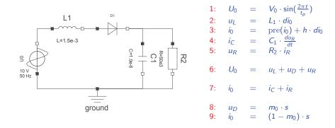
$m_0$  is a discrete state variable. It is *true*, when the diode is *blocking*.
