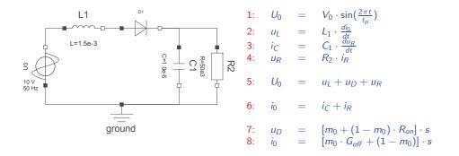
$m_0$  is a discrete state variable. It is *true*, when the diode is *blocking*.
