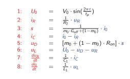
We were able to causalize all equations at once. The system feels like an *index-0* system. However with an ideal diode, we would be confronted with a *conditional index change*.
