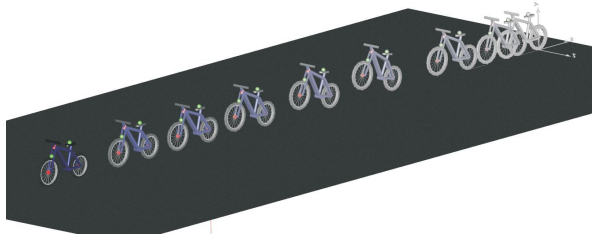
Figure 19: A bicycle with non-ideal tires accelerated by a torque on the rear tire, with the front tire lifting from the ground.
