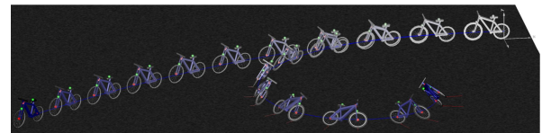
Figure 17: Two similar bicycles with non-slipping tires differing in their geometric properties. The upper bicycle is equipped with ideally slim tires, whereas the lower one driving a narrowing curve has a belted tire with a width of 2cm.
