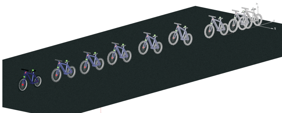
Figure 6.8: A bicycle with non-ideal tires accelerated by a torque on the rear tire, with the front tire lifting from the ground.
