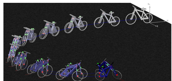
Figure 18: Two similar bicycles with slipping tires differing in their frictional properties. The one driving the inner circle is equipped with the Advanced Friction class, whereas the outer bicycle is equipped with the Dry Friction with Constant Roll Resistance class.
