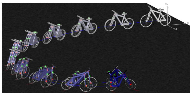
Figure 6.7: Two similar bicycles with slipping tires differing in their frictional properties. The one driving the inner circle is equipped with the Advanced Friction class, whereas the outer bicycle is equipped with the Dry Friction with Constant Roll Resistance class.
