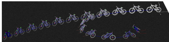
Figure 6.6: Two similar bicycles with non-slipping tires differing in their geometric properties. The upper bicycle is equipped with ideally slim tires whereas the lower one has a belted tire having a width of 2cm.
