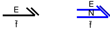
Figure 8.4: The single impulse bond and its multibondgraphic representative. These elements are not part of the standard bond notation.
