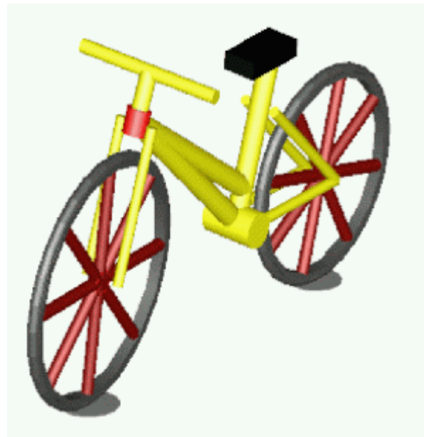
Figure 11: Geometric model of the bicycle
