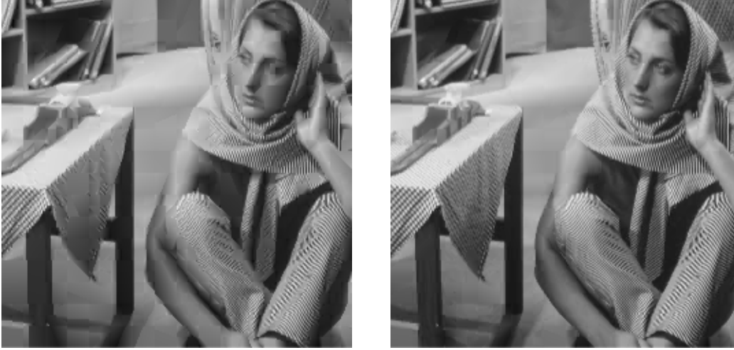
FIG. 5.2. Barbara , 256 \times 256 . Model with 8 possible angles. Left: Linear model, 14730 coefficients, PSNR: 27.79 dB. Right: Linear model, combined with a generic sine model, 14511 coefficients, PSNR: 33.29 dB.
