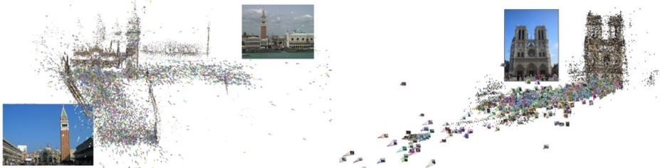
Figure 9: Left: 3D reconstruction of the San Marco Dataset with 10338 cameras. Right: Reconstruction from the Notre Dame dataset with 1300 registered cameras.
