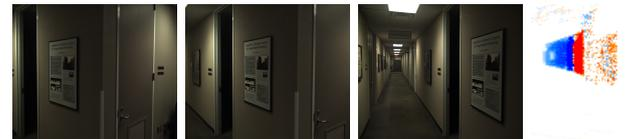
Fig. 11. Input images showing the hallway junction. The floor and ceiling are not observed in some region in the junction. Also the wall on the opposite site is not observed. The last image shows a vertical slice of the occupancy grid. The floor, ceiling and left wall are missing only the right wall is shown in red, which means a positive weight.
