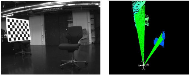
Fig. 7. The chessboard and the chair as seen on the left are marked as candidate obstacles in the virtual scan shown on the right.
