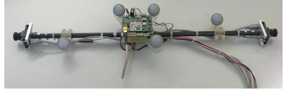
Figure 6. The stereo rig used during the experiments.
