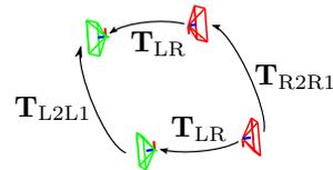
Figure 3. Rig constraint linking the euclidean transformations.
