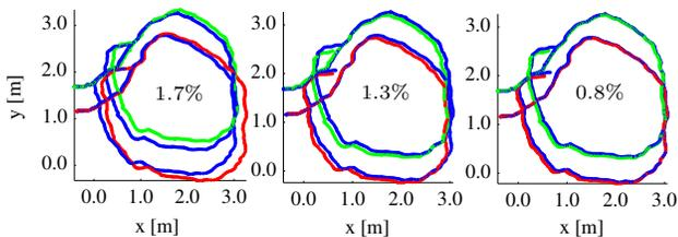
Figure 8. Dataset 'Circle' with different algorithm configurations:  $(\bar{S}, \bar{F})$ ,  $(S, \bar{F})$  and  $(S, F)$  with drifts. The ground truth is colored in blue, the motion estimates are red (right) and green (left).
