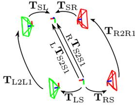
Figure 5. Transforming camera motions to rig reference system.
