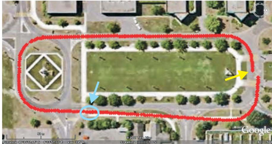
**Fig. 7.** The estimated path (before loop closing) superimposed onto a Google Earth image of the test environment. The scale is shown at the lower left corner. The cyan arrow indicates the position of the three road humps. The yellow arrow indicates the starting position of the vehicle.
