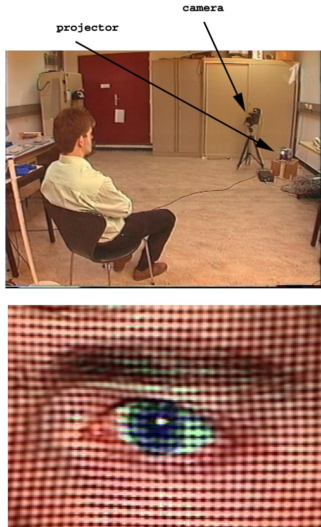
**Figure 3. Top: The active system only consists of a normal slide projector and camera, and a computer. Bottom: A regular square pattern is projected on the scene, as seen in this detailed view.**
