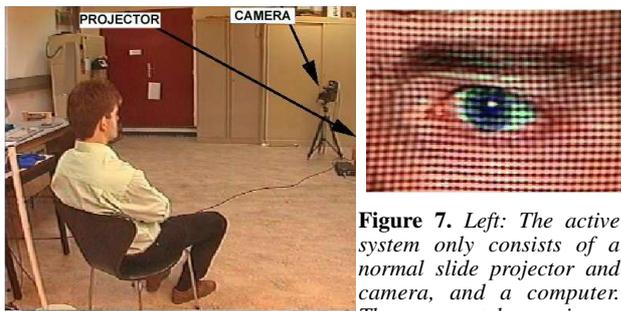
**Figure 7.** Left: The active system only consists of a normal slide projector and camera, and a computer. The camera takes an image from a direction that is slightly different from the direction of projection. Top: A regular square pattern is projected on the scene, as seen in this detailed view. In this case, the grid covers the complete face. 3D co-ordinates are calculated for all the line intersections, resulting in the simultaneous measurement for thousands of points.
