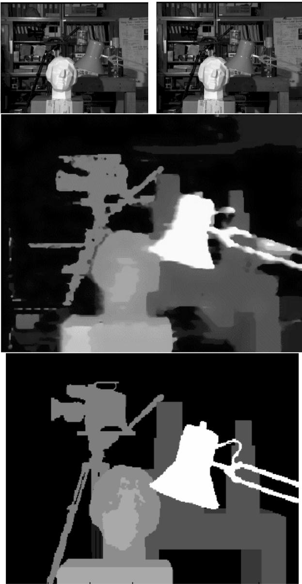
Figure 11: Tsukuba dataset for testing accuracy. Original left and right image are shown at the top. The disparity map is presented in the middle. The ground truth can be found at the bottom.
