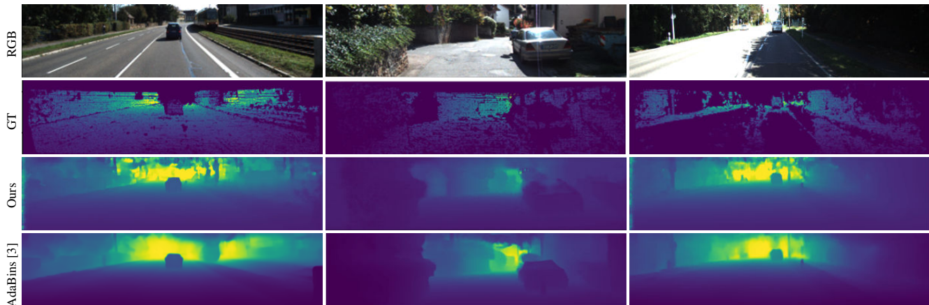
Figure 3: Qualitative predictions on the KITTI [18] dataset. We show the performance of NVS-MonoDepth (Ours) compared to AdaBins [3] leading to similar predictions, but with a much simpler architecture. Color scale: 0 (purple) to 80 meters (yellow).
