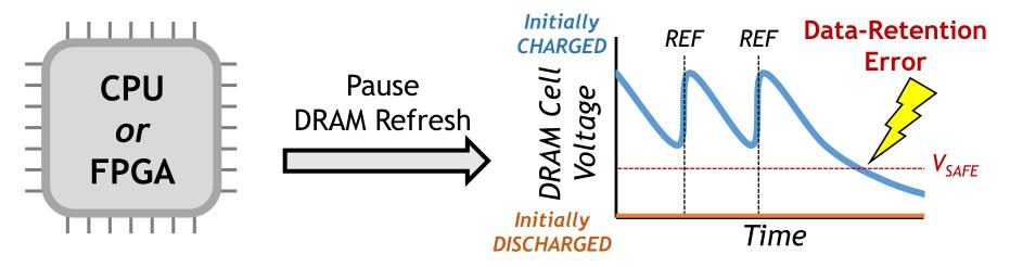
Difference between CHARGED and DISCHARGED cells allows us to restrict errors to specific bit positions
