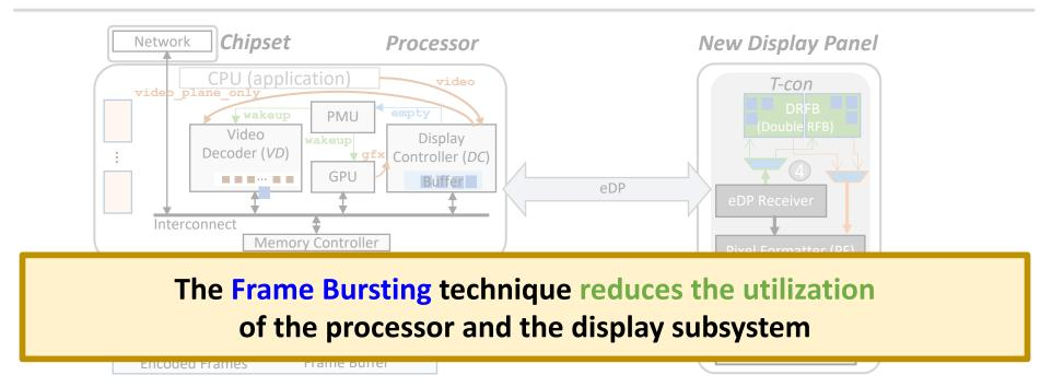
The system can enter deep low-power states between bursts for transferring the decoded frame from the DC to the remote frame buffer
