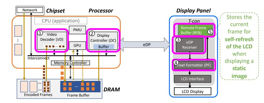
A conventional display subsystem consists of five main components:
