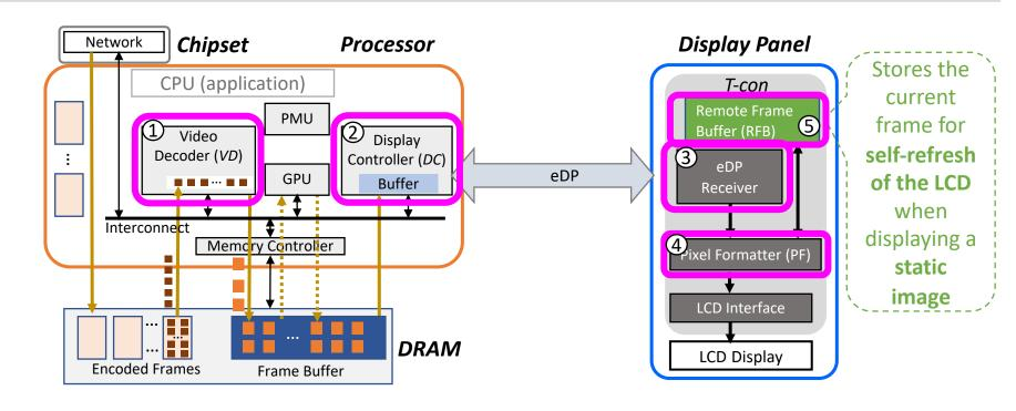
A conventional display subsystem consists of five main components:
