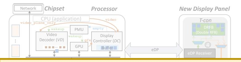
Frame Buffer Bypassing reduces the energy consumption of the host DRAM by eliminating unnecessary data movement to/from the DRAM frame buffer
