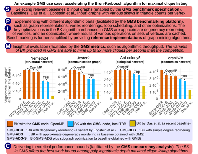
Figure 1: Performance advantages of the parallel Bron-Kerbosch (BK) algorithm implemented in GMS over a state-of-the-art implementation by Das et al. [42] and a recent algorithm by Eppstein et al. [51] (GMS-DGR) using a novel performance metric “algorithmic throughput” that shows a number of maximal cliques found per second. Details of experimental setup: Section 8.
