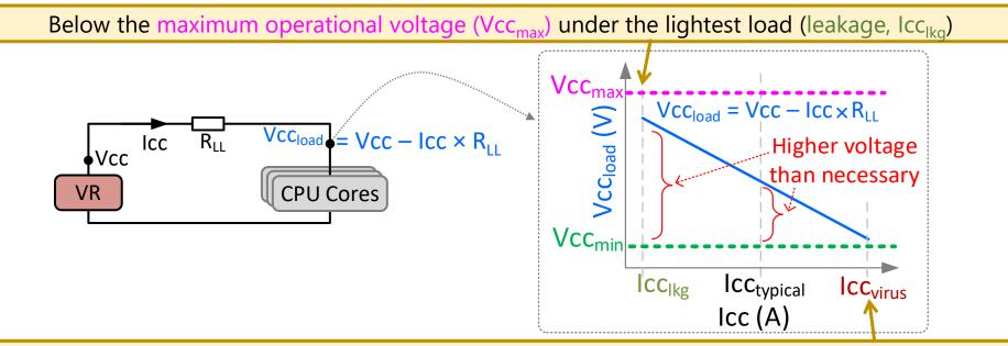
Above the minimum functional voltage (Vcc<sub>min</sub>) under the most intensive load (power-virus, lcc<sub>virus</sub>)
